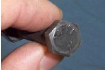
This bolt on the left is small but incredibly strong. It's markings are clear even after some years of operation in a car. It is also has a fine thread making it a UNF Grade 8 bolt. I actually know for a fact what this bolt is, due to having regularly replaced many of the components it holds in a car over the last 20 or more years.
