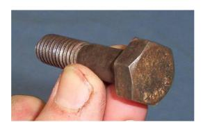
This is bolt below is looking better, typical Grade 5 bolt markings on the top face of the head of the bolt, so it should be either a UNC or UNF bolt and much stronger than the first two shown.
