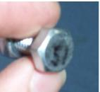
While the photo of the bolt on the right almost looks like an automotive bolt because of it's recessed area on top, but as it has no markings so we can only deduct it is a standard home hardware available, Grade 4 bolt. Most probably witworth [BSW British Standard Witworth] thread also.
