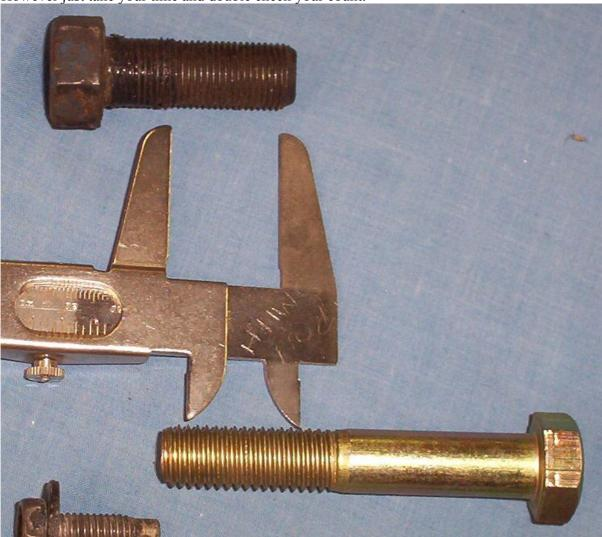
The top bolt is 5/8 inch diameter with 18 threads per inch so it will be UNF.
