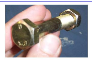
Now this is more like it, clearly marked as a 10.9 strength metric bolt. This bolt is a bolt that is offered to bolt the tow ball coupling casting to front draw bar on a trailer.
