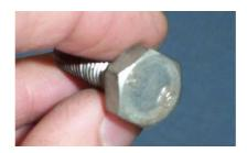
This bolt above is an interesting one. It has the 'M' symbol but no numbers. The 'M' indicates this is definitely a metric bolt, however because it has no number markings we have to assume it is a low grade general purpose bolt. Other low grade metric bolts may not have the M but display their 4.8 grade rating instead.
