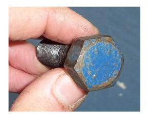
Before this one goes back it will get some assistance in the form of some 'Lock Tite' solution on the threads to ensure it never comes loose again until I want it to. It is common for Grade 8 UNF bolts to also be referred to as a 'high tensile bolt'.
