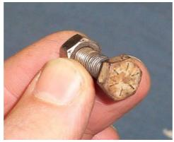
Three of these bolts locate the lower ball joint in the suspension arm on all Ford Falcons and the like from about 1969 to 1989. Another two larger grade 8 bolts assist them and attach the front radius rod to this lower suspension arm. Obviously a suspension arm is a highly loaded area, so the Original Equipment Manufacturer [OEM] replacement part has opted for the strongest bolts they can put in and opted for a fine threaded bolt to minimize the chance of the bolt working it's way loose.
