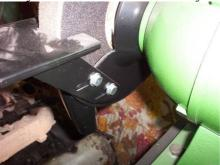
This picture below shows a hand operated bar bender with the handle fixed to it using two metric 4.8 low grade bolts.
