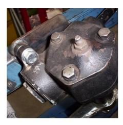
Here is the steering box – held in by grade 8 UNF bolts
