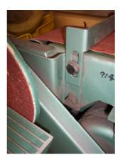
The example above is on a linisher, while the example below is a pedestal grinder. There are no head markings on these bolts and they are installed in a relatively loss stress applications.
