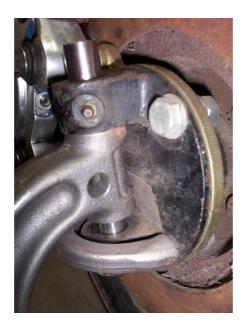
Here is the disc brake caliper bracket held in place by grade 8 UNF bolts.
