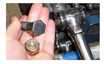
Shown here is the part of the front beam axle suspension from my hot rod project. All the components are aftermarket all supplied from 'Rod City Repros'. Look at the main bolts that hold the front radius rods to the batwing. Oversized for their application 5/8 grade 8 UNF bolts
