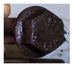
This is a grade 8 bolt. It is a standard Cleveland engine bolt that holds the cylinder head to the engine block.
