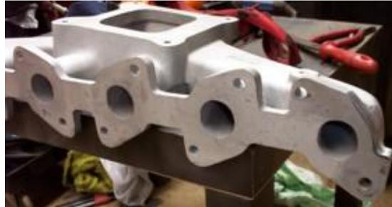
So there you have it the finished manifold ready for fitting above and two close up pics from above and below on how the manifold now clears the shape of the back of the water neck housing.
