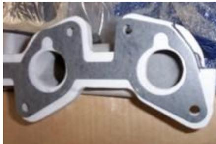
Use this marked up gasket to pen mark the manifold as to how far it needs to be taken down.
