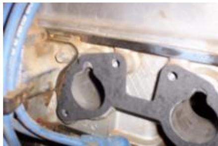
The photo above shows how close the water neck is to this front inlet port, use the standard gasket to measure off. Place some pen marks on the gasket where the location of the water neck housing is close to the gasket. This will be your guide as to how much needs grinding off the front lip of the inlet manifold.
