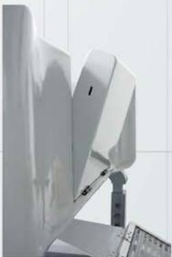
Fiberglass Foldable Door, Playing The Role of Step Ramp
