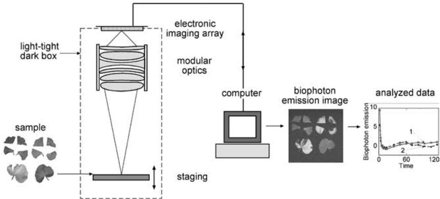
Fig. 1. Schematic of biophoton imaging system.
