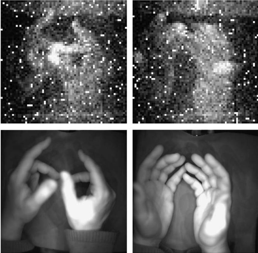
Fig. 10. Top images are 10-minute exposures taken in total darkness using  $20 \times 20$  binning with a Princeton Instruments VersArray 1300B camera cooled to  $-100^{\circ}\text{C}$ . Bottom images are 10 ms exposures taken with white-light illumination.
