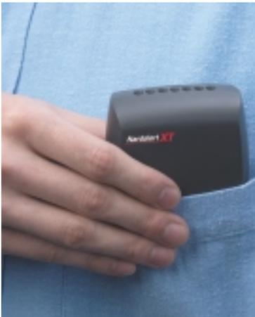
Nardalert XT is a handy warning device that is ideal for your breast pocket. It comes with two types of clip that allow you to either wear it in a shirt pocket or on a belt. One of the two optional soft cases attaches to a safety harness such as those used by climbers. The **< warning lights >** are located on the top front side and are therefore easy to read at a glance.
