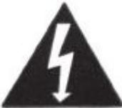
This “bolt of lightning” indicates that uninsulated material within your unit may cause an electrical shock. For the safety of everyone, do not remove product covering.
