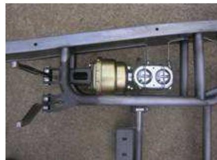
The pedals come standard polished S/S and are fixed to a cast pedal mount that is incorporated into the centre X member. The pedals have a S/S pedal pad pivot on top of them that allow you to position your pedal pad to where you like it and then tighten to fix it. This is a unique feature only available on the Lakes components.
