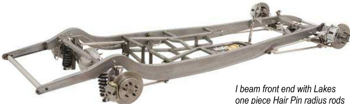
*I beam front end with Lakes one piece Hair Pin radius rods*
