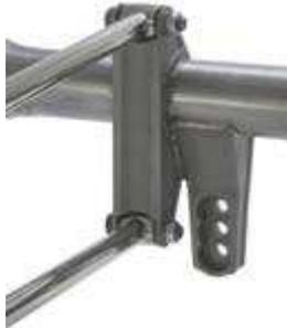
Another feature that comes standard with the Lakes product is that where ever there is the underside of a nut or bolt, there is a raised surface so that they are not tightened up onto large painted surfaces. This is a huge advantage over previously fabricated bracketry where the bolt and nut actually affected the whole face of the bracket's painted surface.
