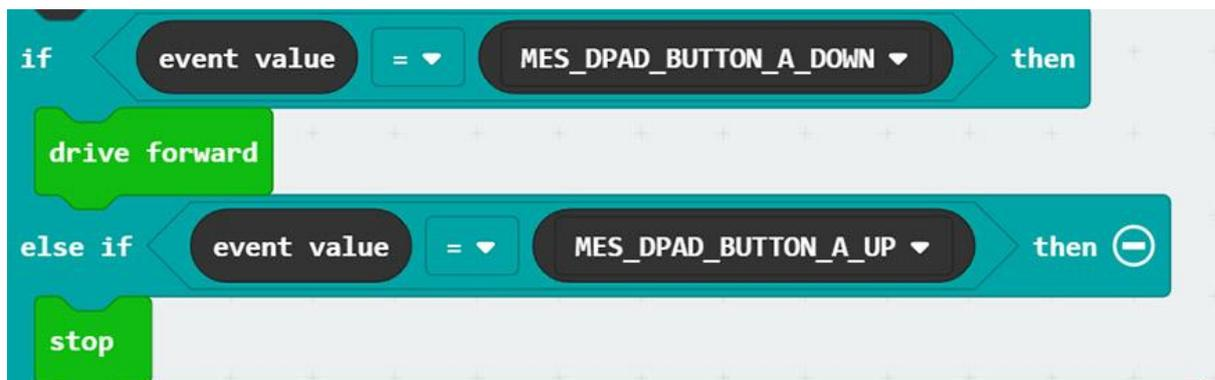
In the code above you can see how the code for the A button press works. When the A button is pressed, the buggy will drive forwards. When the A button is released, the buggy will stop.
