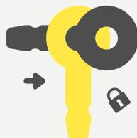
Push the leg **all the way through** the head to lock in place. The connectors are limited in rotation.
