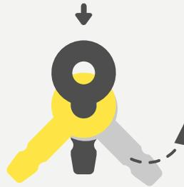
Push the leg all the way through to create a joint with limited movement.
