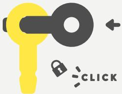
Slip the head into the groove of the leg and **listen for the click**. This will secure connectors and allow rotation.
